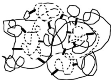
Figure 8. Schematic diagram of a model of mixing in the blends. The thin solid line represents polystyrene, the dotted line represents poly(ethyl acrylate), and the thick solid lines represent the interactions between sulfonate and pyridine groups.
